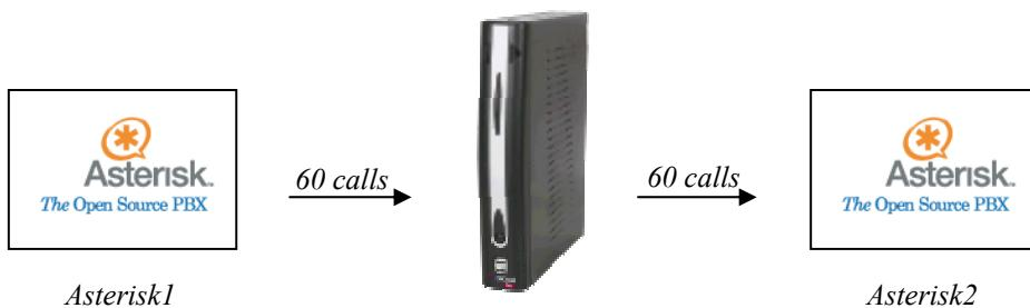
*The Asterisk on the left generates a call into the TS-1, and the TS-1 forwards the call to the Asterisk on the right. The TS-1 serves as a gateway between 2 SIP networks.*
